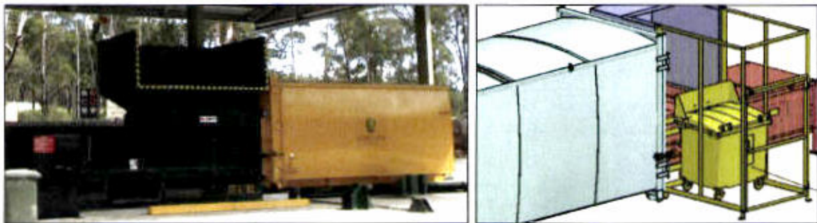
Figure 3-5: Example of a compactor unit and sealed hook lift bin & Bin Tiler for compactor
